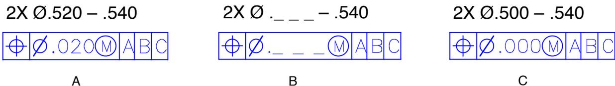
**Figure 7-19 Converting a positional tolerance of a hole to a zero positional tolerance**
