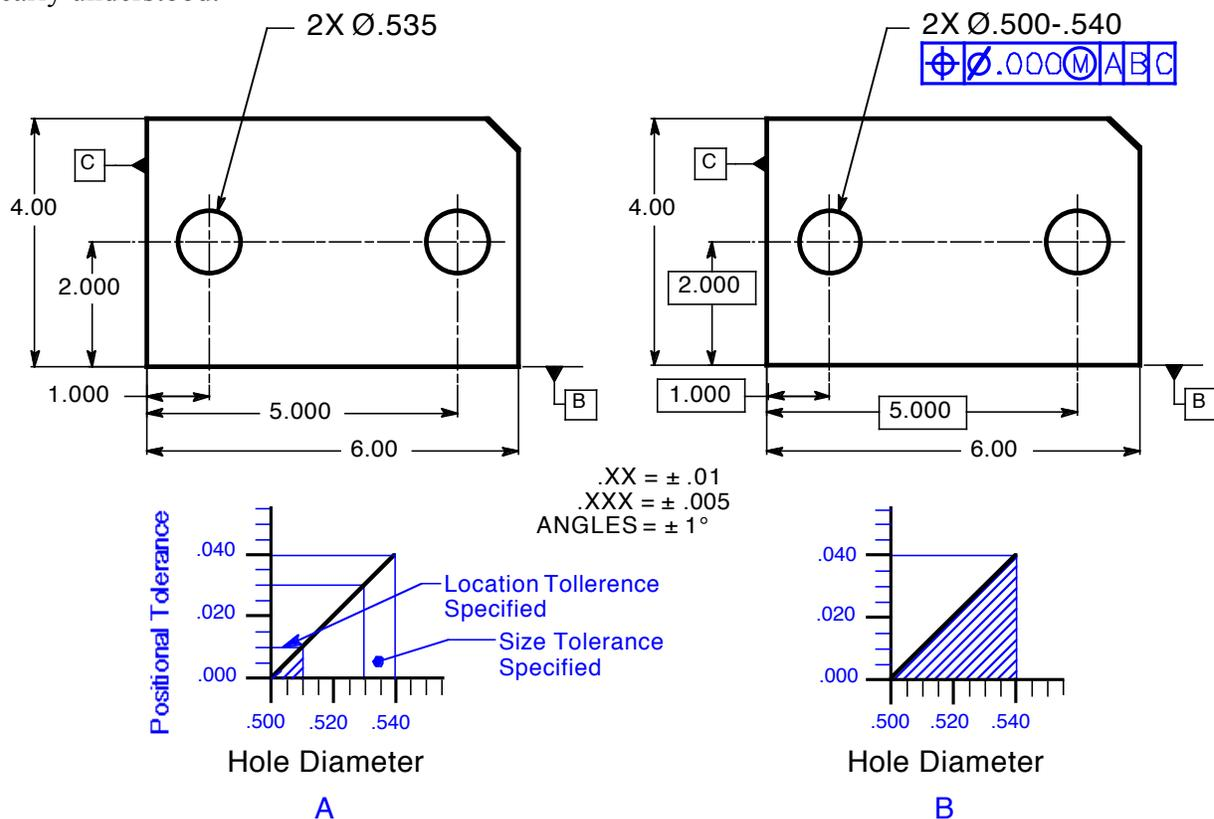
**Figure 7-17 Plus or minus location tolerance compared with zero positional tolerance.**
