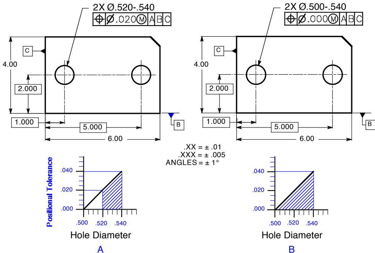
**Figure 7-18 A specified position tolerance compared with zero positional tolerance.**
