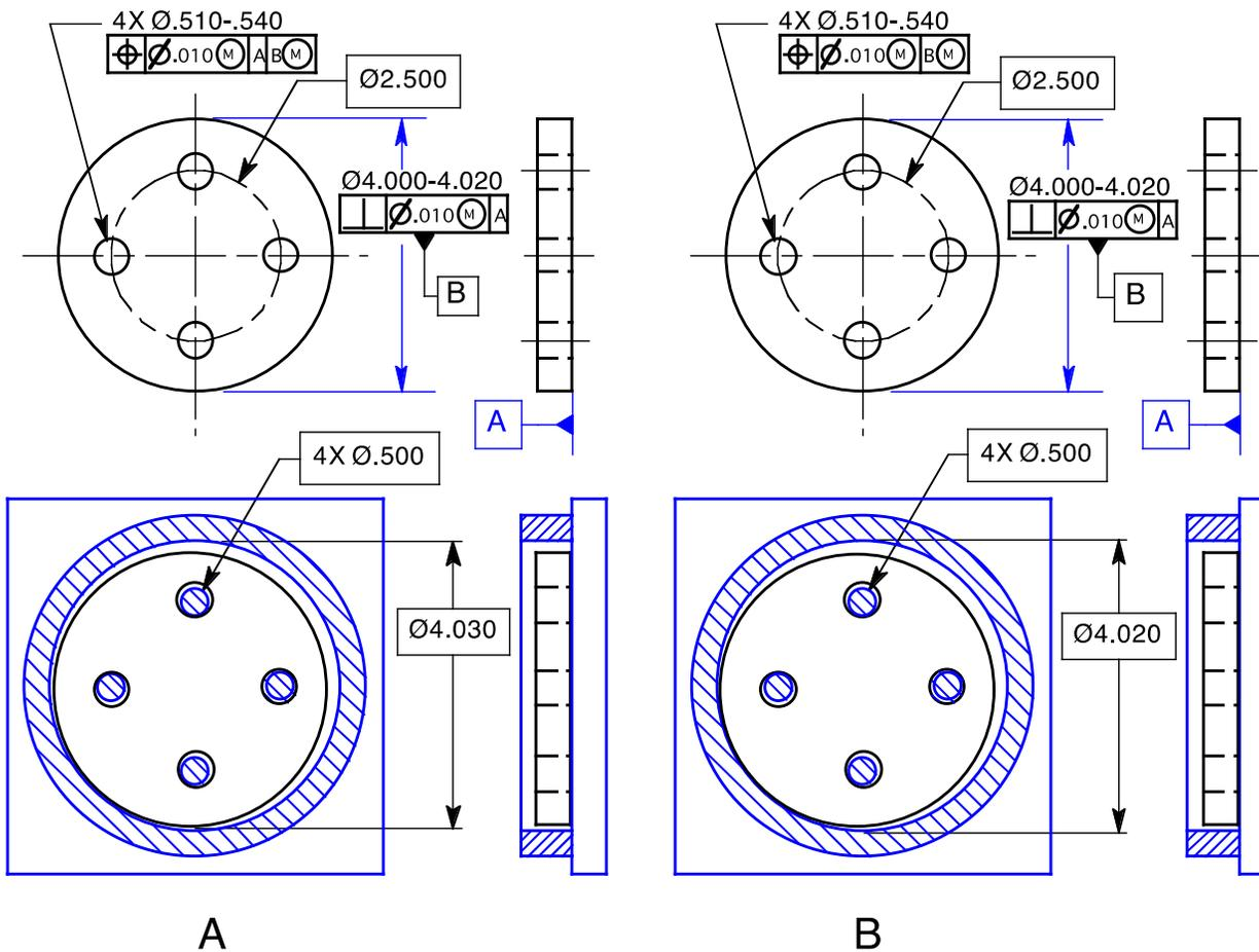
**Figure 7-8 Inspection of a hole pattern controlled to a datum feature of size at MMB**
