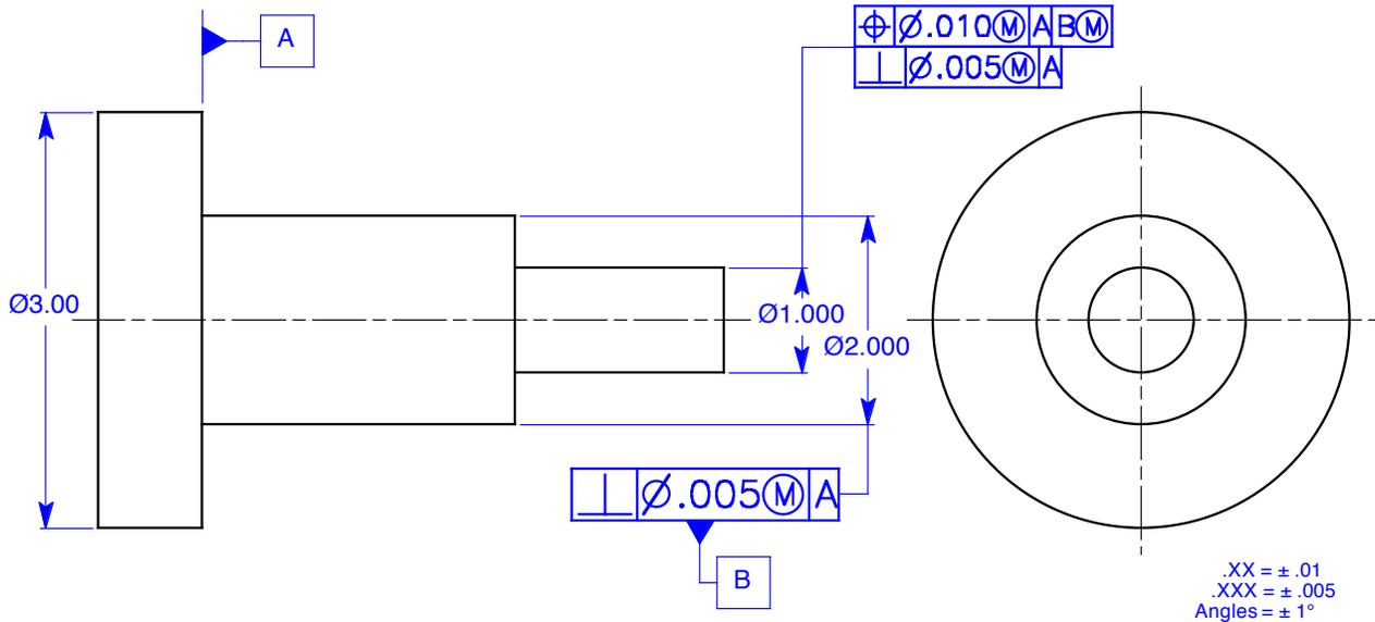
**Figure 6-4B** The properly toleranced part shown in Fig. 6-4A
