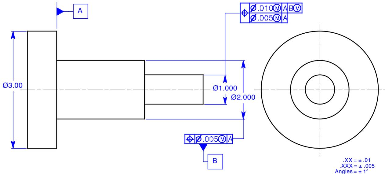
**Figure 6-4A The inappropriate use of the position control to control perpendicularity**
